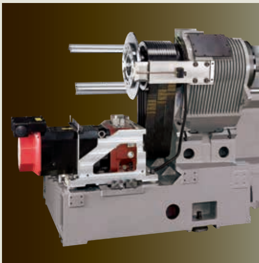
C-axis by belt-driven spindle with gearbox
