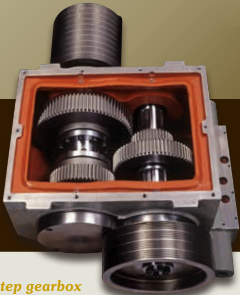
C-axis by belt-driven spindle with gearbox
